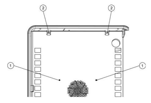
Figure 5-4 Removing the Air Baffle
