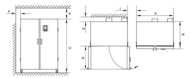
Figure 3-3 Floor stand incubators, dimensions and required clearances
