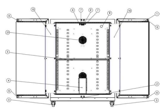
Figure 4-7 Heratherm IMH 750-S Front View
