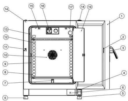
Figure 4-1 Heratherm IMH 60/ IMH 100/ IMH 180 Front View
