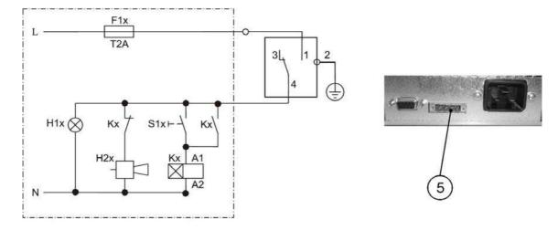
Figure 5-11 Alarm Contact Connection Example
