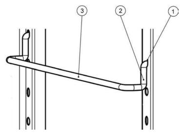
Figure 5-8 Shelf Support Bracket Installation
