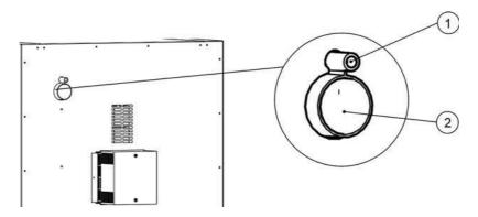
Figure 4-12 Connecting Nozzle for Fresh-air Filters (Accessory Item)
