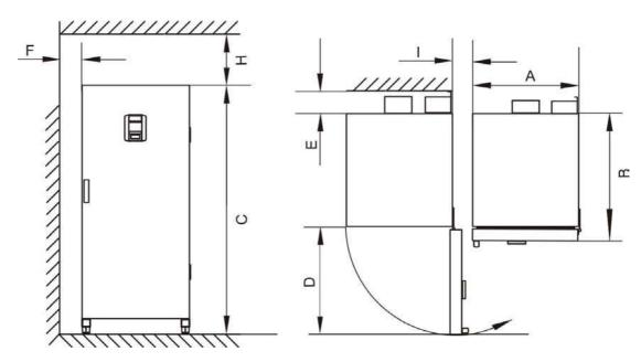
Figure 3-2 Floor stand incubators, dimensions and required clearances
