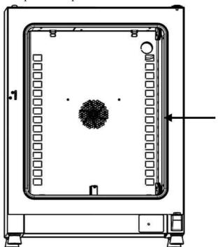
Figure 10-1 Door Seal Replacement
