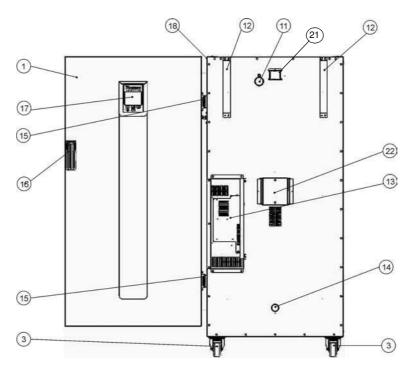
Figure 4-6 Heratherm IMH 400-S Rear View
