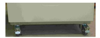
The floor stand incubators come equipped with four (4) casters. The lever for releasing the caster is located above the locking lever. After positioning the unit in its installation location ensure that the locking levers are pressed down on the casters.
