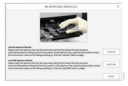
Figure 91. Aperture loading instructions screen.
