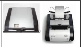
Figure 109. Positioning the Injector System on top of the GloMax® Discover System.
