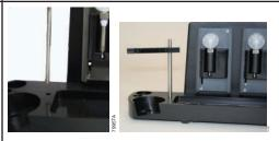
Figure 111. Inserting the vertical support rod and inlet tube holder.
