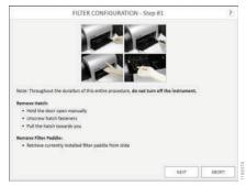
Figure 82. Filter Configuration procedure.
