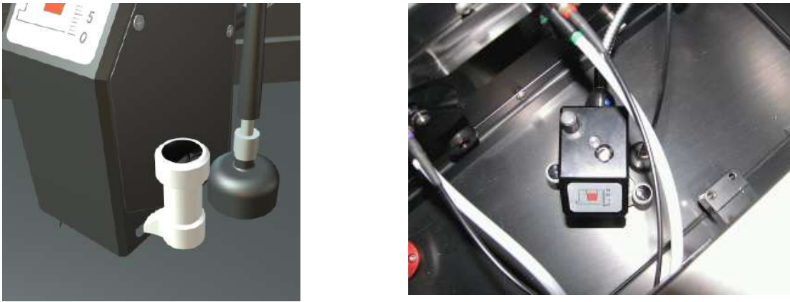
Figure 22: Schematic of the Quick-Fix holder (left) and actual image of the TRF-optic head in the instrument (right).
