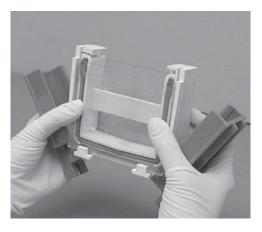
e. The arms of the clamping frame push the short plates up against the notch in the green gasket, creating a leak-proof seal. At this point, the sample wells can be washed out with running buffer, and sample can be loaded.
