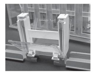
c. Lift the gel sandwiches or cassettes into place against the green gaskets. Make sure the Mini-PROTEAN 3 short plates sit just below the notch in the gasket.
