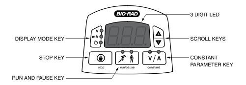
Fig. 3. Front Panel.
