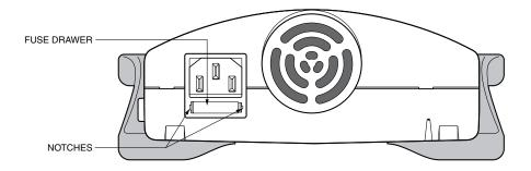
Fig. 5. Rear View Showing Fuse Drawer with Notches.
