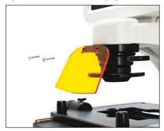
Secure the UV shield in place
