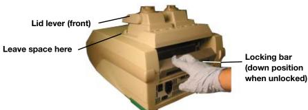
Figure 4. Inserting the reaction module into the bay.
