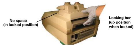
Figure 5. Locking the reaction module in place.
