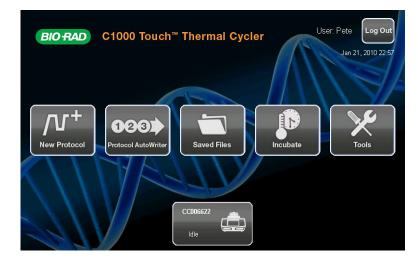
Figure 8. The home screen of the C1000 Touch thermal cycler.
